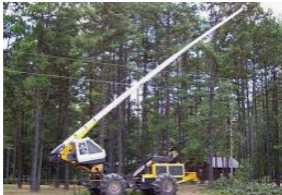
The Jarraff operator was intending to trim a small branch from the side of a larger branch located at a height estimated to be approximately 18m from ground level. As he was operating the Jarraff with the boom extended the wind blew the larger branch against the cutting blade.
