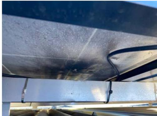
Result of a poor crimp under the array
