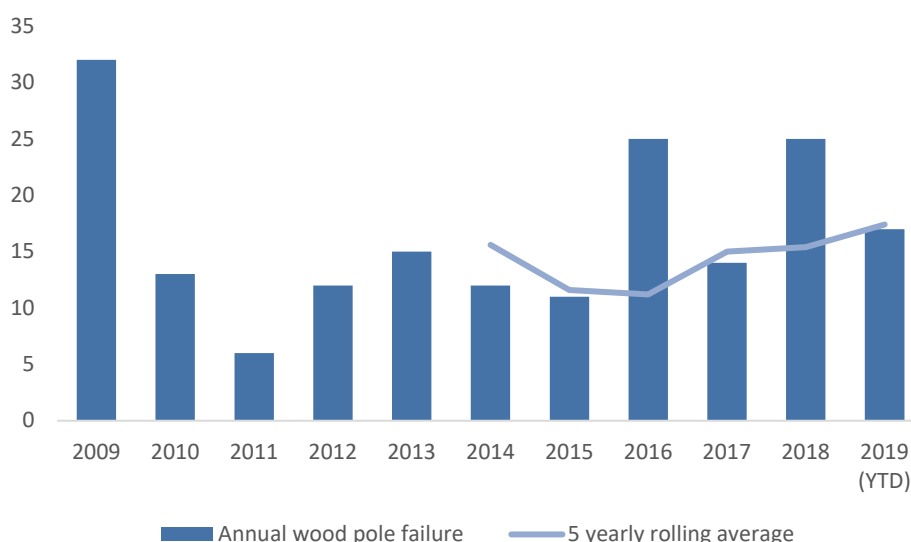
Figure 6 Powercor's wooden pole failures
