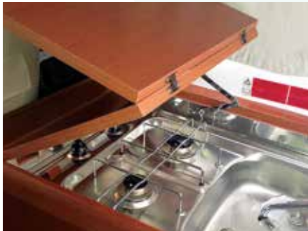
Figure 8: Stowed gas appliance
