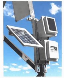
LineVision uses LIDAR and EMF sensors plus digital twinning analytics to spot power line movement and damage that could ignite wildfires.
